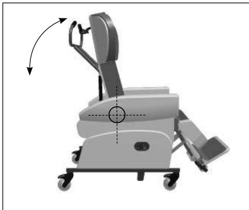
Back Angle Recline (BAR), where hip angle can be adjusted.
