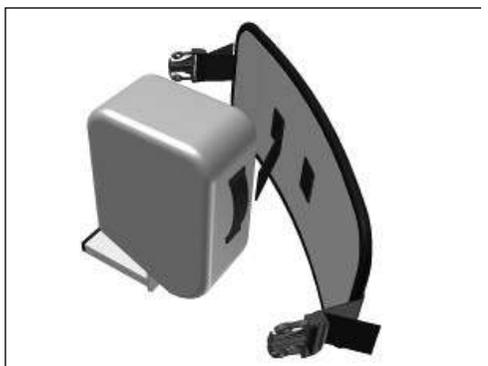
Fit the tab on the inside face of the knee strap through the loop on the front of the pommel.
