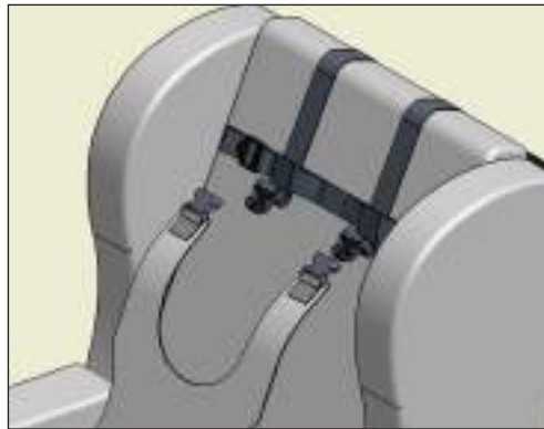
Four point harness to provide support to the upper trunk.
