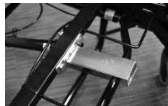
Pommel bracket fitted to front cross tube of seat frame.
