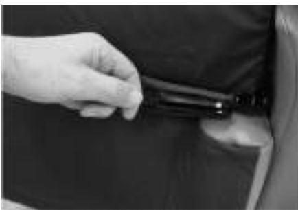
Separating the two halves of the crumb catcher which joins the seat to the legrest.
