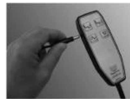
Connecting the 24V DC charger to the motorised SmartSeat handset.
