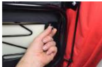
Remove the flange nut at each corner of the middle cushion wire to remove the middle cushion.
