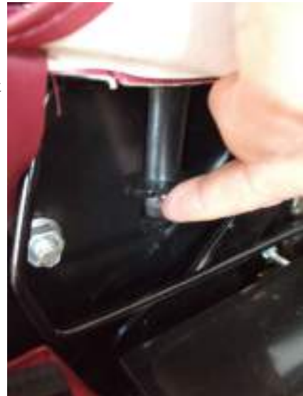
Depress the button to release the front arm mounting peg.
