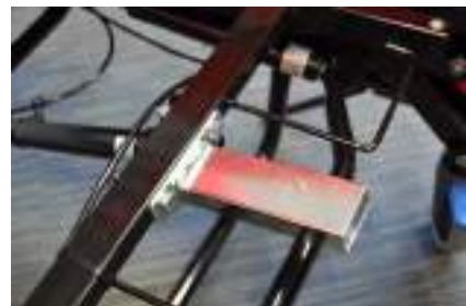
Pommel bracket fitted to front cross tube of seat frame.
