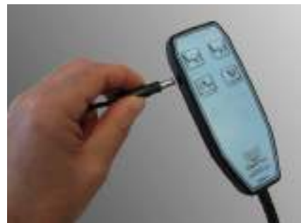
Connecting the 24V DC charger to the motorised SmartSeat handset.
