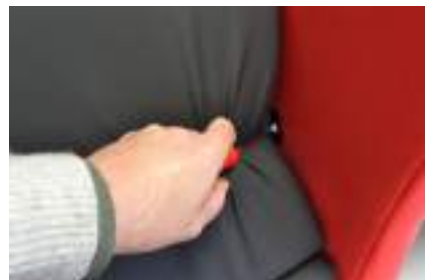
Use a 5mm ball end allen key to loosen the second from top wing mount.
