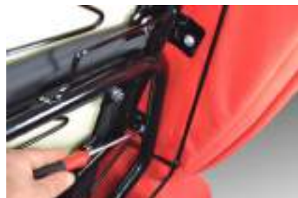
Remove the valance and undo the two lower wing mounts with a 5mm ball end allen key.
