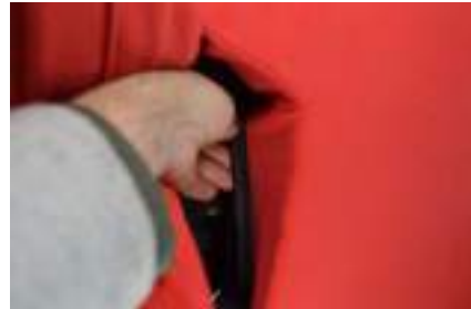
Grip the 'J' strip at the top and un-clip from the thin side bar.
