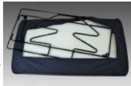
Wire pulled out sideways.
