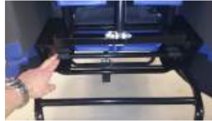
For Back Angle Recline, the straps mount on the round bar at the rear of the BAR base frame.
