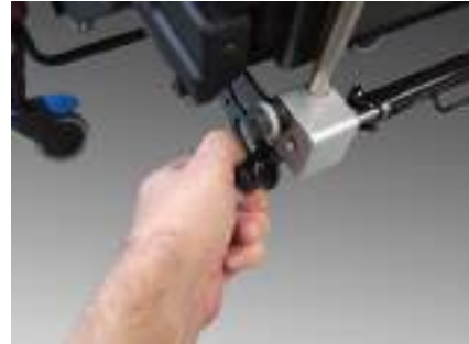
Pull out the round knob on each side of the back edge of the footplate to adjust footplate angle.
